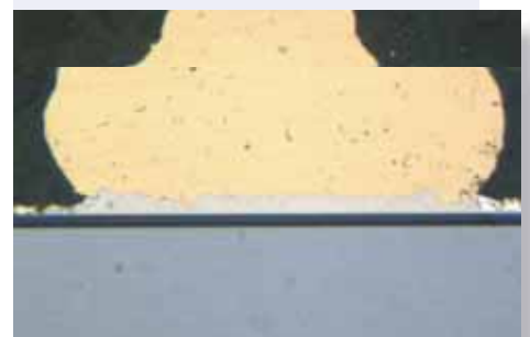
Fig. 12b: Detail: Au-ball-bond (diameter 20µm); Al-metallization consumed by intermetallic phase growth
