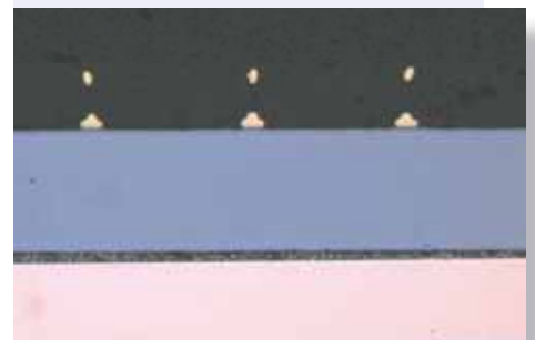
Fig. 12a: Overview: Thermally cycled Si Chip joined to lead frame with conductive adhesive - Au ball bonds on Si Chip
