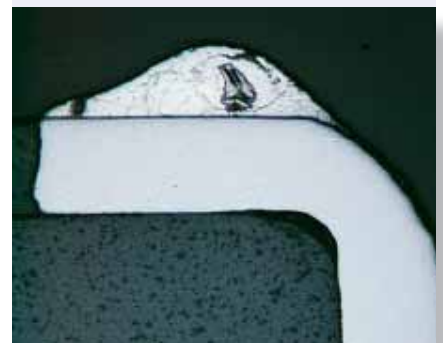
Fig. 4: Sample 2 ground with Diamond Pad 20 µm
