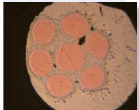
Fig. 19: SnAgCu 1.3 – lower dissolution rate because of copper saturation in solder alloy (1000x)
