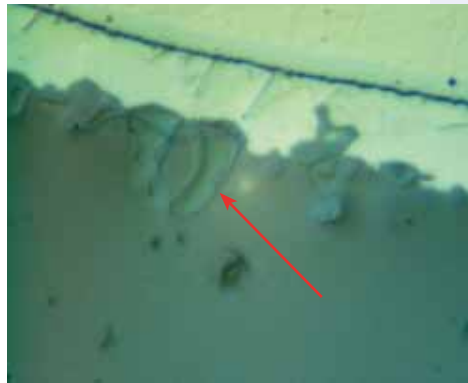
Fig. 23: Microsection of jelly cap whisker (1000x)
