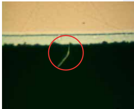
Fig. 21: Microsection of tin layer with grown whisker (preparation plane measured with optical measuring station)
