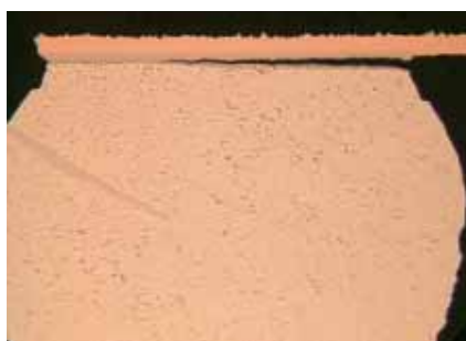
Fig. 15: Brittle fracture after thermal cycling (1500x)
