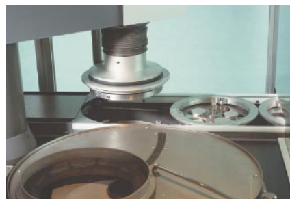
3. The specimen holders are collected from the conveyer belt, using a special lifting device
