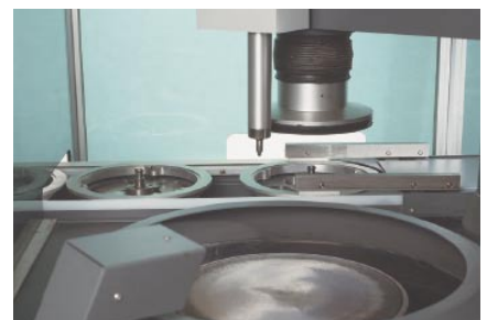
7. The finished specimen holder is moved to the conveyer belt, where it can be collected by the metallographer for microscopic examination
