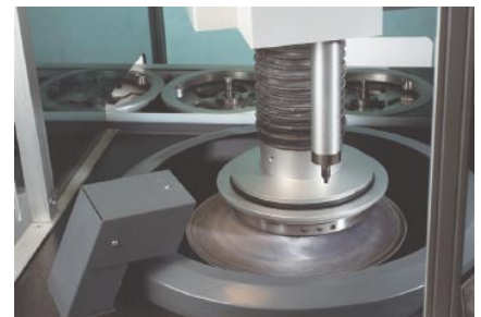
6. After fine grinding the specimen holder moves on to polishing
