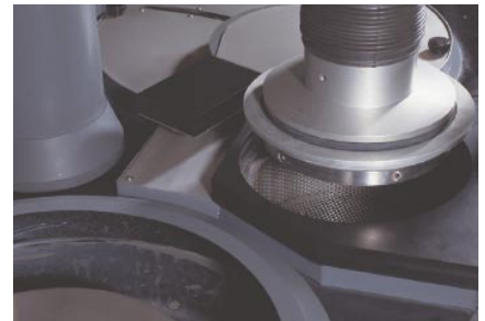
5. When the grinding is completed, the specimen holder is carried to the cleaning chamber
