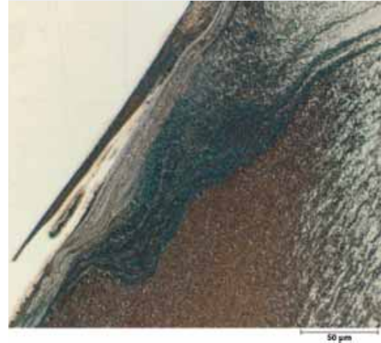
Fig. 5: Image of the lower part of the damaged region (etchant: Nital)
