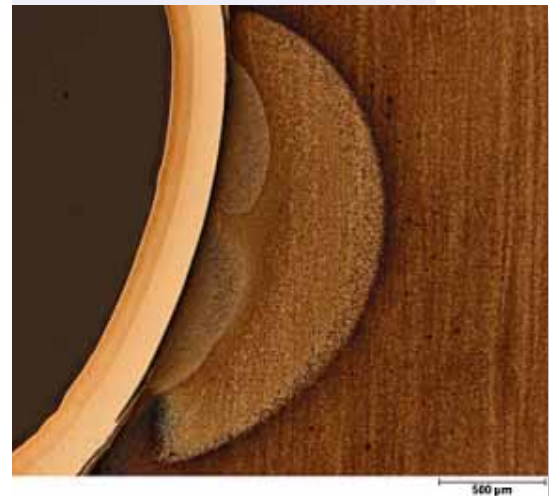
Fig. 6: Low-magnification optical microscopy image of the damaged region (etchant: iron(III)-chloride)
