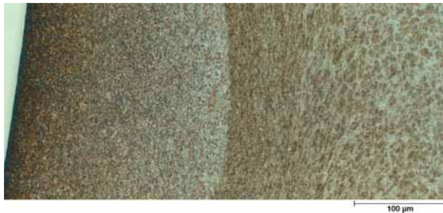
Fig. 7: Detailed image of the damaged region (etchant: iron(III)-chloride)
